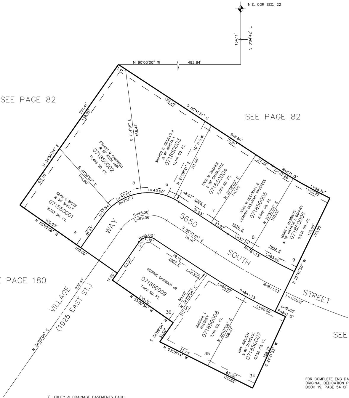
7' UTILITY & DRAINAGE EASEMENTS EACH SIDE OF PROPERTY LINES AS INDICATED BY DASHED LINES EXCEPT AS OTHERWISE SHOWN.
